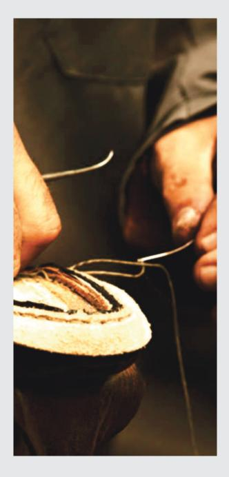
Goodyear welting is the oldest, most labor intensive, and most durable of the three methods of construction. It can be done by machine or by hand and involves multiple steps.
